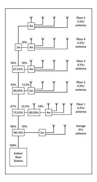
To make the most of the benefits of coaxial DAS systems, it is very important to minimize loss at every stage and have the bandwidth to cover present and future needs. For economic reasons, both send and receive signals share the same cable. The system must be designed for the optimal Transmit and Receive levels at every antenna location. This requires very careful planning. A combination of equal and unequal signal splitters establishes the same path loss between base station and each antenna.
